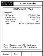
Note: A temperature bath at  $25.0 \pm 1.0$  °C is required for this measurement.
