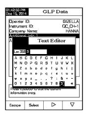
Press Escape to return to the GLP Data options. If the Saving Confirmation is enabled, press to accept the modified option, No to escape without saving or Cancel to return to the editing mode. Otherwise, the modified options are saved automatically.
